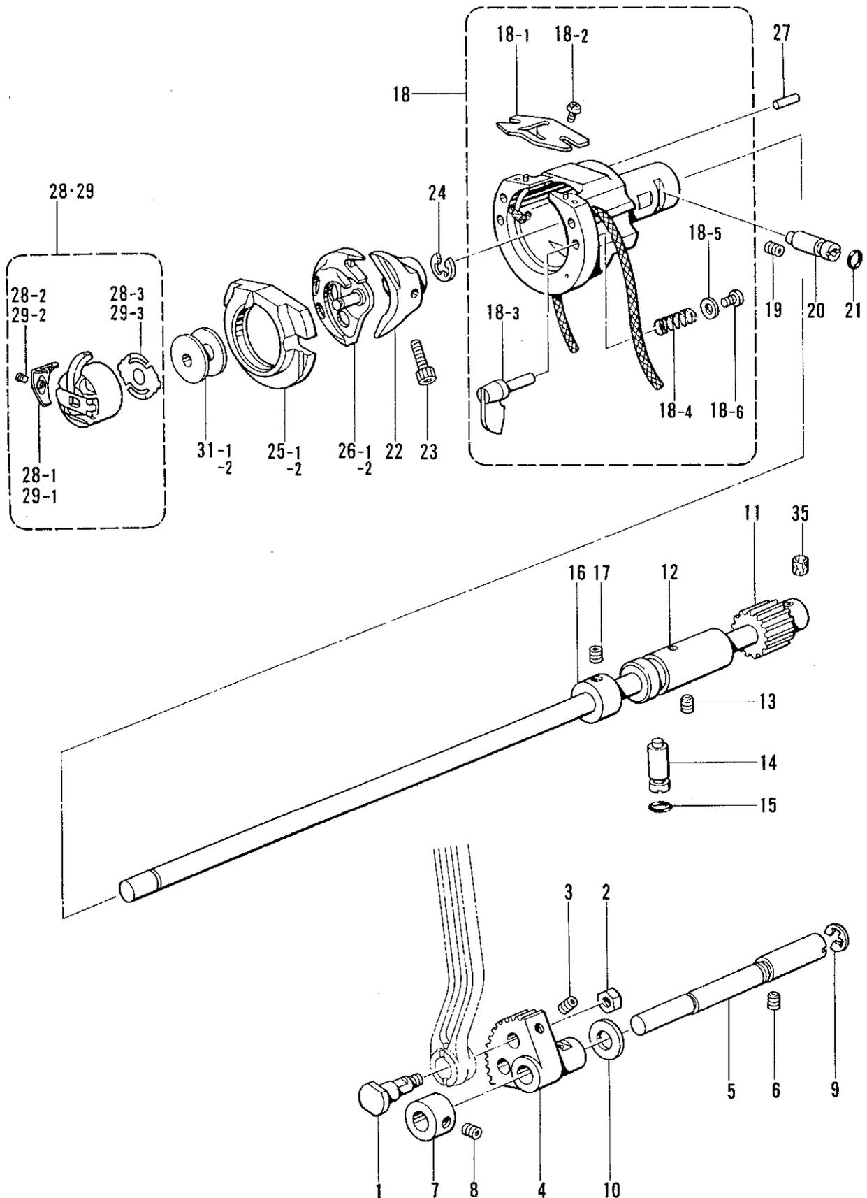
F. 下軸関係/Lower shaft mechanism/Untere Welle/
