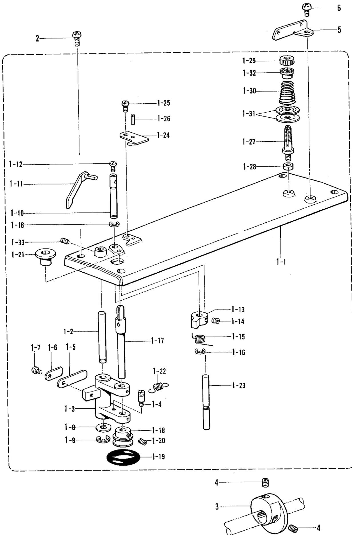
J. 糸巻関係/Bobbin winder mechanism/Spuler/
