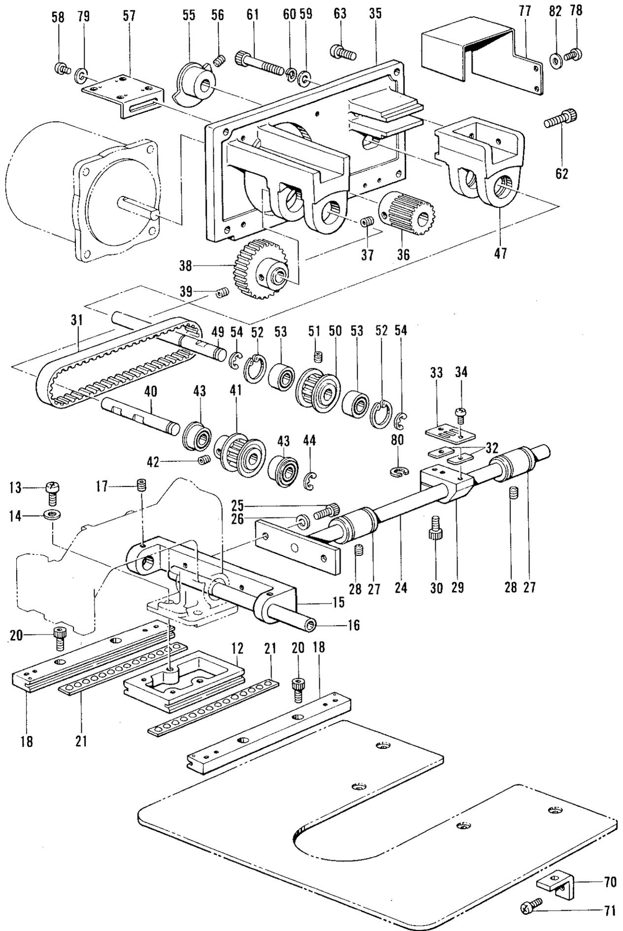
C. 送り関係/Feed mechanism/Transportvorrichtung/
